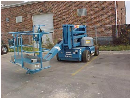
Figure 7. Bucket lifts can provide a safer and more efficient way to work in high areas.
