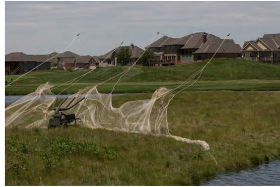
Figure 24. NetBlaster™ in mid-launch. Photo by Stephen M. Vantassel.
