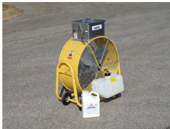
Figure 10. Methyl anthranilate may be dispersed using a large fan. Photo by Stephen M. Vantassel.
