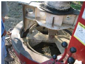
yoke out of ring gear
